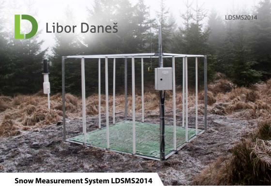
An accurate and highly reliable device for measuring of snow water equivalent (SWE) on the weighting principle. The device is accompanied by a mechanism minimizing the possibility of measurement errors by snow bridging. It can be easily completed by measurement of snowmelt seepage and many other characteristics of environment.
